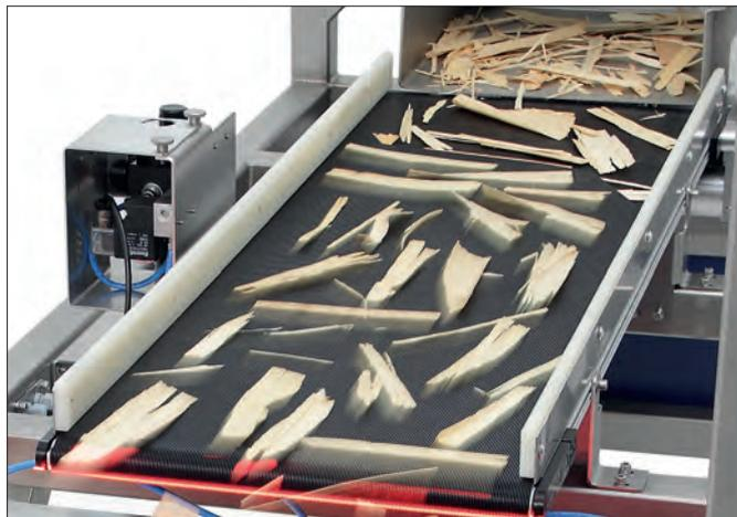
HAYER CPA 4 CONVEYOR, alignment and separation of longish samples on the conveyor
