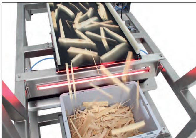
HAYER CPA 4 CONVEYOR analyzing size and shape of wood chips
