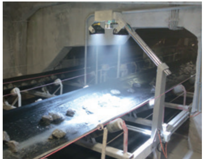
HAYER SOLO M4 for material analysis directly over belt conveyors.
